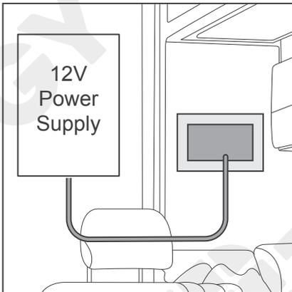
2. Tape the mounting template to the selected mounting location, and measure whether the 12V power cable is long enough to connect Renogy ONE to your DC power supply. If the included 12V power cable is not long enough for connecting Renogy ONE to your DC power supply, re-select a mounting position or use an extension cable ( $\geq 22$  AWG). If you do not need to extend the 12V power cable, go to [Step 5](#).
