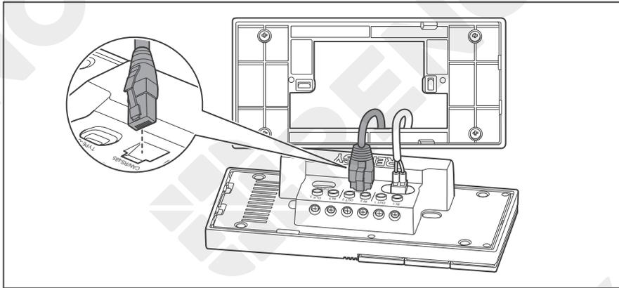
4. Connect the pre-embedded RJ45 connector to the RJ45 port of Renogy ONE.
