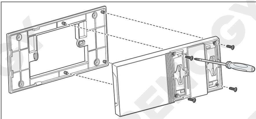
2. Put Renogy ONE on the base, and drive in the four M2 screws with the Phillips screwdriver #1 through the mounting holes to fix the Renogy ONE on its base.
