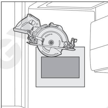
5. Use the drill and skill saw to dig the installation hole according to the gray mark on the mounting template.
