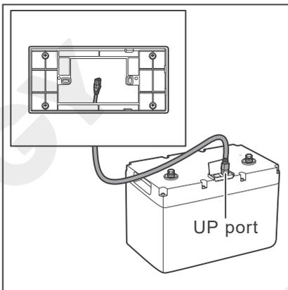
5. If there is only one device, insert the other end of the communication cable to the communication port of the specific device in use.
