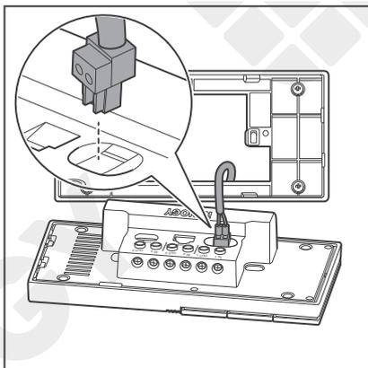
2. Insert the 12V power cable terminal block into Power Port of Renogy ONE.
