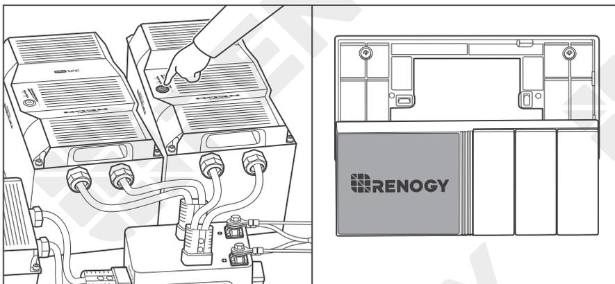
3. Power on the DC power supply and check if Renogy ONE automatically turns on with the LCD lighting up.
