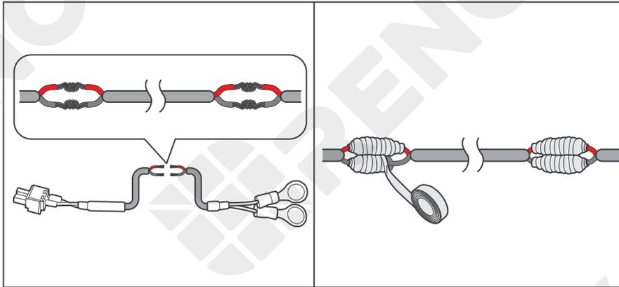
4. Strip some insulation off the extension cable, and connect the cable to the included 12V power supply cable. Tape over the cut-off areas.
