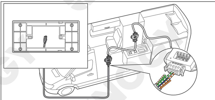
3. Replace the terminated drop tap at either end of the RV-C bus with the Common Drop Tap (not included). Secure the bare wires of the Drop Cable (not included) onto the terminal block plug of the Common Drop Tap following the terminal block plug pinout.
