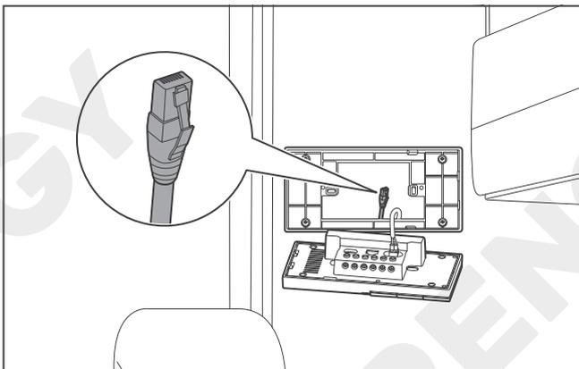
2. Reserve one end of the communication cable into the installation hole.
