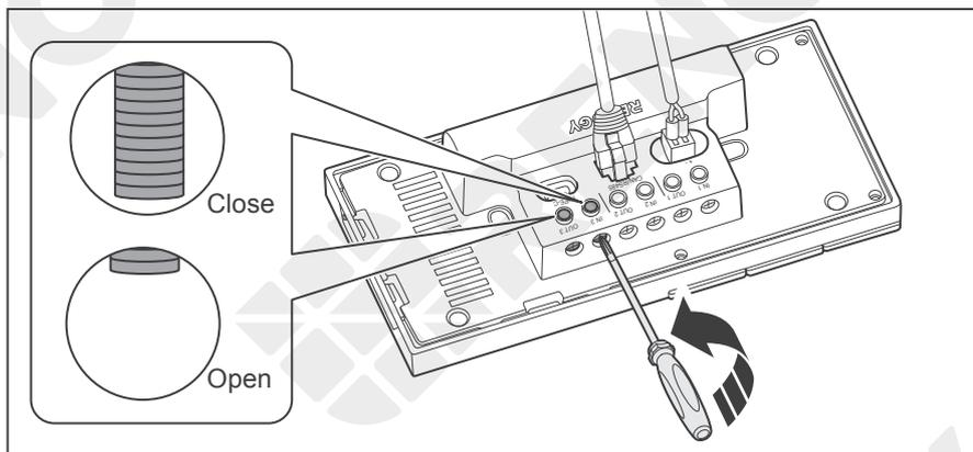
2. Use a Phillips screwdriver to turn the wire hatch screw counterclockwise. Make sure that the terminal hatch is completely open.
