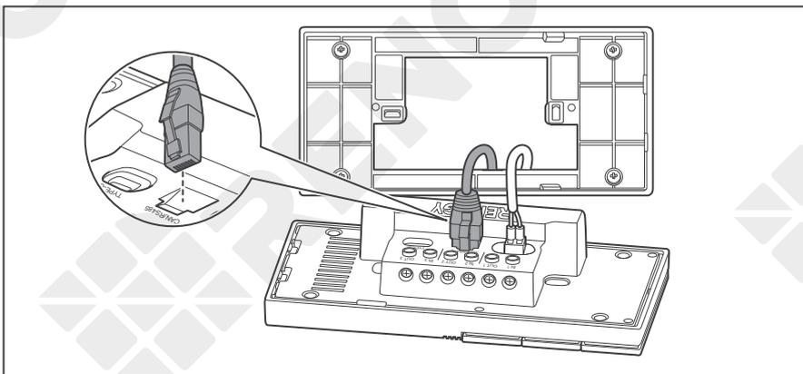
5. Connect the pre-embedded RJ45 connector to the RJ45 port of Renogy ONE.
